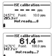
Position the sachet to ensure sensor membrane and ceramic junction are completely immersed in solution. A value close to 100 ppm and the message "Not ready..." will be displayed.
