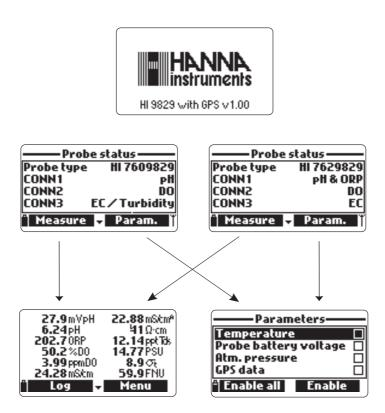
The probe status screen identifies the probe and attached sensors. Non-logging probes are identified as **HI 7609829** and logging probes are identified as **HI 7629829**.
